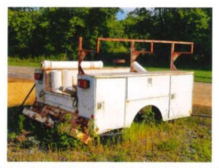
2. This trailer has been used by many departments over its time in Jonesborough. It has a walking beam chassis under it that is very worn out, there are no parts available to repair it, it also needs brakes all the way around, And all wheel bearings and seals. The tires are worn out as well. This trailer when turned sharp, the tires rub the frame, this causes the trailer to run sideways behind truck that is towing it.
