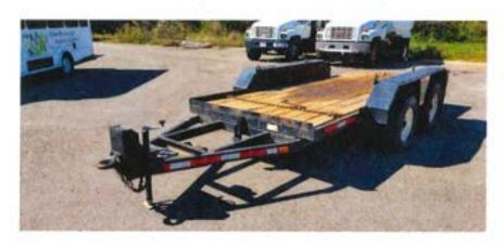
This trailer has bearing failure that has damaged the spindles on both ends of axles. It uses mobile home tires and rims which are illegal for anything except mobile home or farm use. It needs brakes. It needs axles. Its tongue is bent. This trailer is small and under rated for transport of most of our smaller excavating equipment.
