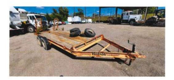
4. This 20,000lb rated trailer has been here for 28 years. Needs: tires, axles, brakes, new decking, paint job and rewired. Would be a lot cheaper to buy one new.
